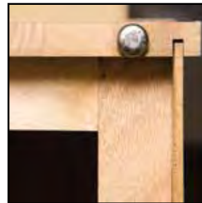
Full Length Back Panel with 1/4" Dado Minimum 3/4" Wood Sides
