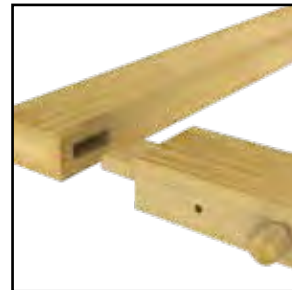
Mortise & Tenon Joint Frame
